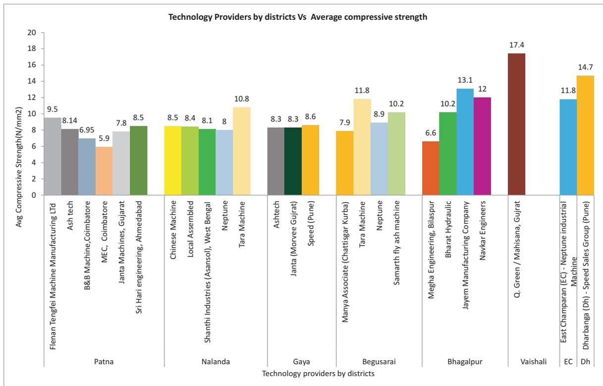
Figure 14: Technology providers and their average compressive strength
