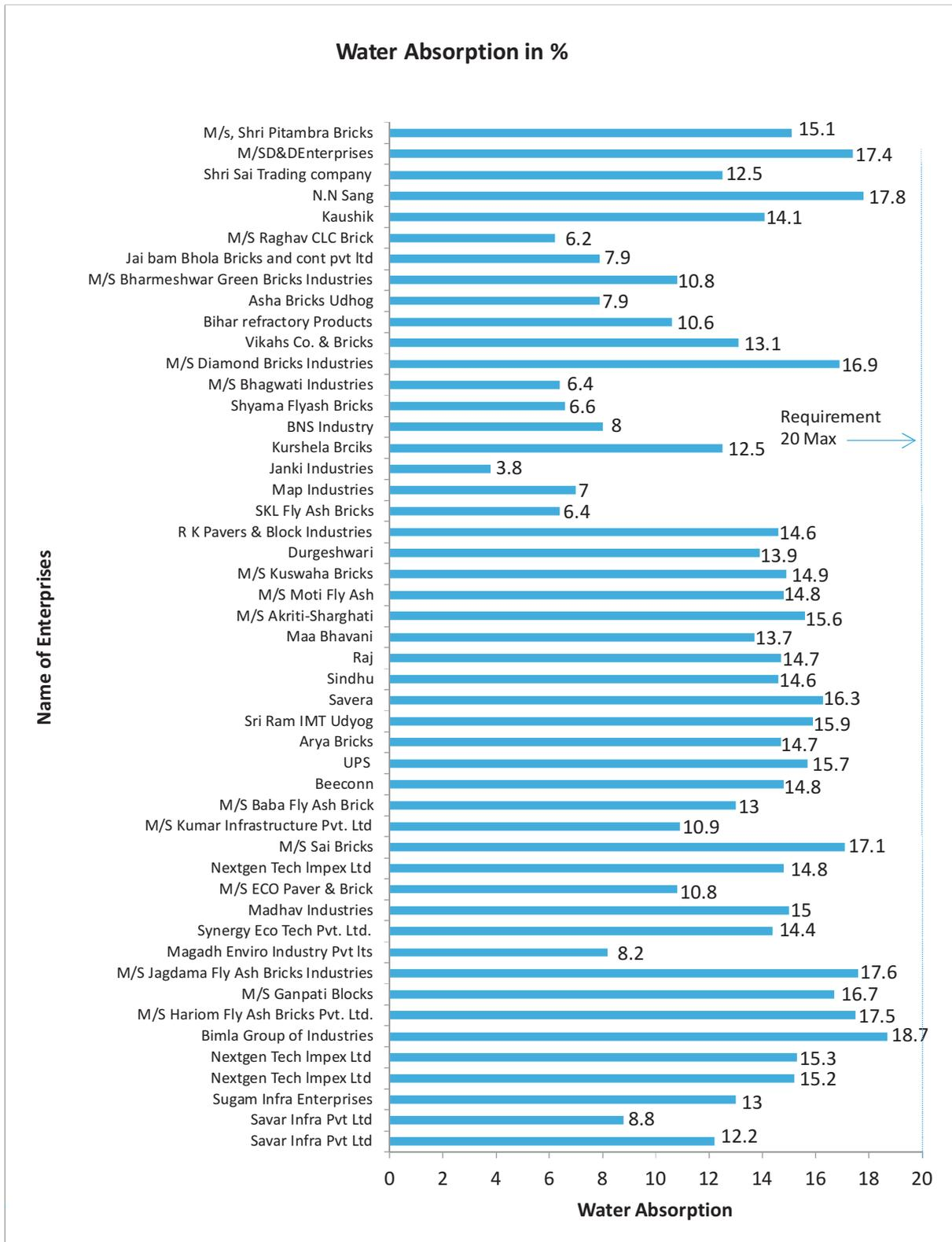
Figure 19: Graph on quality testing results – Water Absorption
