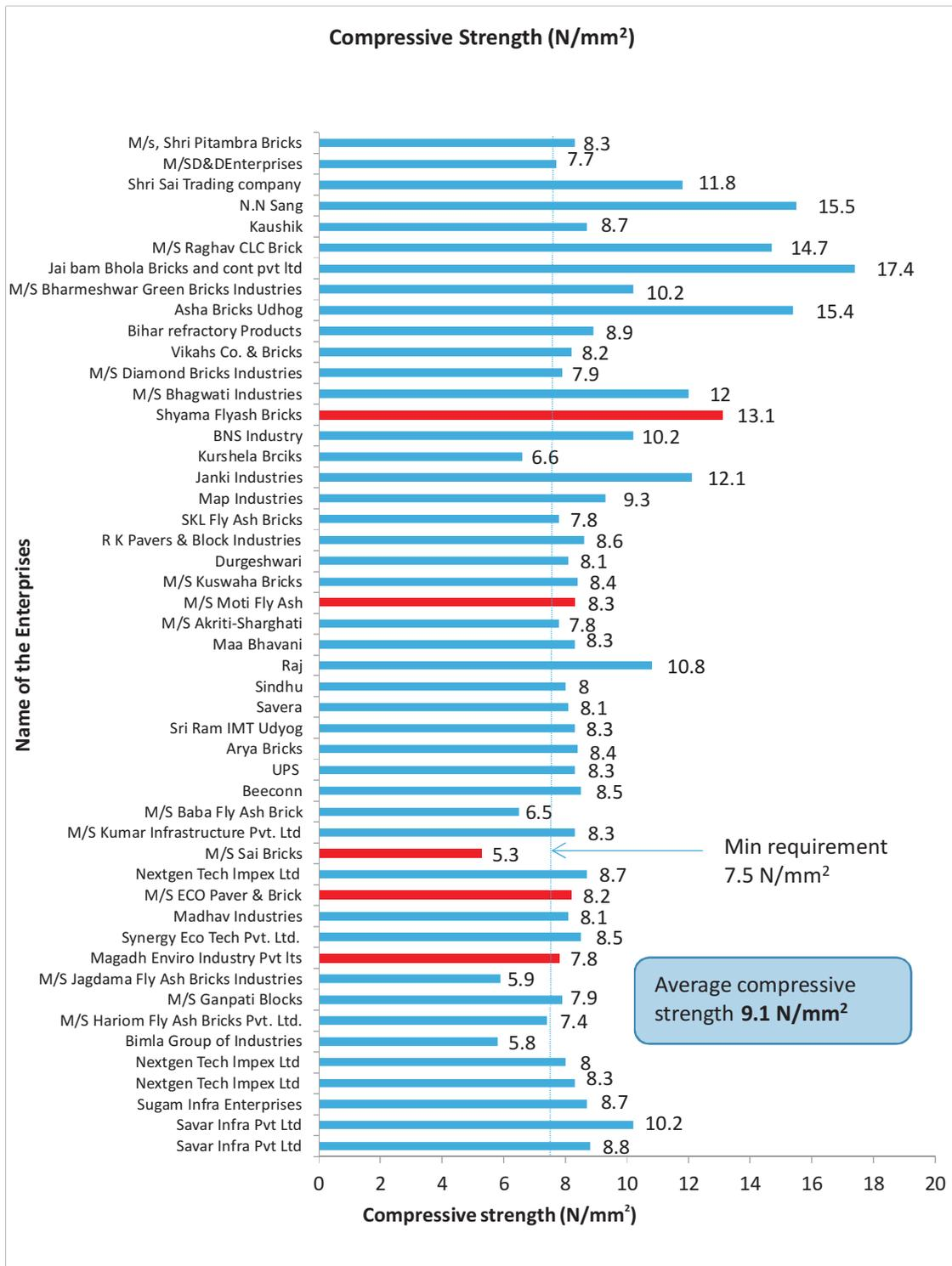
Figure 20: Graph on quality testing results – Compressive strength
